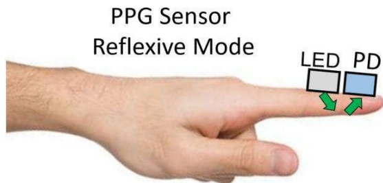
Fig. 1. PPG sensor in reflexive mode
