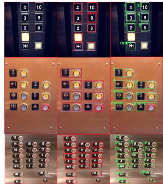
Fig. 11. Elevator Button Label Recognition. (a) Input images. (b) Ground-truths of button detection. (c) Results of button recognition.
