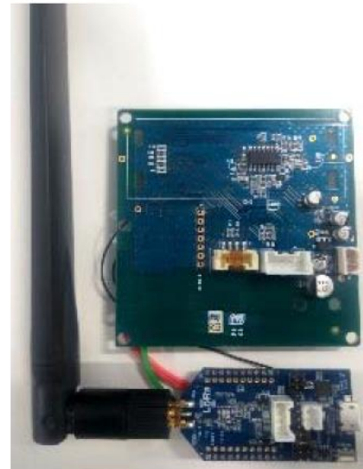
Figure 4 Fault Indicator with LoRa module
