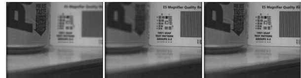
(a) Image 1 (Focus on left) (b) Image 2 (Focus on right) (c) Fused Image (All focus)
