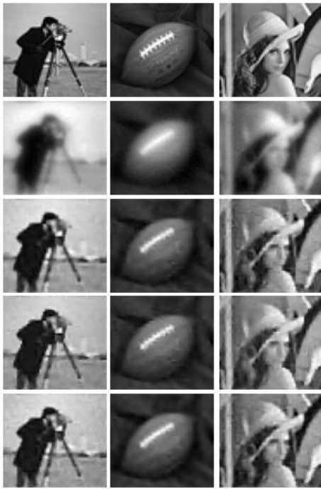
Fig 10: Original resized 60 \times 60 cameraman, football and Lena images (First row), their blurred versions (second row), Restored images using: SSF-SESOP (third row), PCD-SESOP (fourth) and IRLS-SESOP (fifth)
