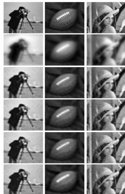
Fig 9: Original resized 60 \times 60 cameraman, football and Lena images (First row), their blurred versions (second row), Restored images using: SSF (third row), SSF-LS (fourth) PCD-LS (fifth) and IRLS-LS (sixth)
