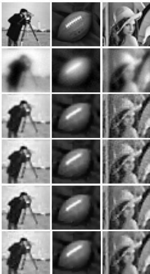
Fig 7: Original resized 40 \times 40 cameraman, football and Lena images (First row), their blurred versions (second row), Restored images using: SSF (third row), SSF-LS (fourth) PCD-LS (fifth) and IRLS-LS (sixth)
