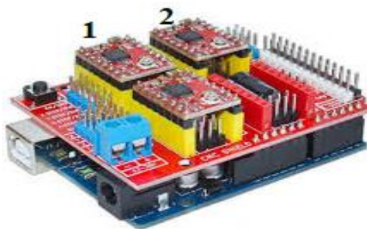
Fig. 9: Stepper Drivers with CNC Shield Connection
