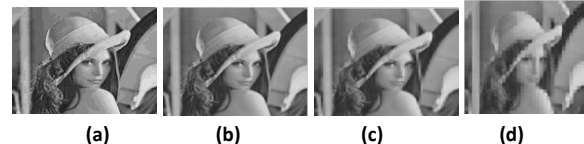
Fig.1 BTC Result (a) Original Image (256 x 256) (b) Reconstructed Image (4x4) (c) Reconstructed Image (8x8) (d) Reconstructed Image(16 x16)
