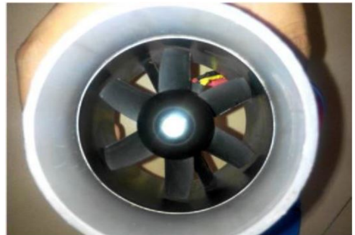
Fig. 8. Suction cup with ducted propeller.
