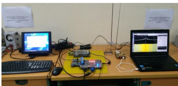
Fig 18: An experimental test case of FPGA/DSP based HF transceiver
