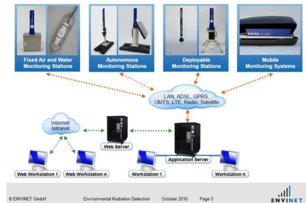
Fig. 2 RDMS network structure designed by Envinet (Envinet, 2017)
