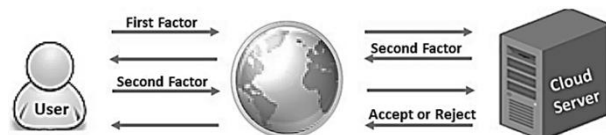
Fig 1: Principle of 2FA in cloud computing [23].
