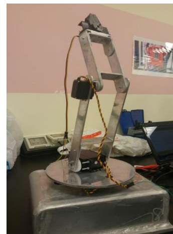
Figure 8: The manufactured 3 DOF robotic arm
