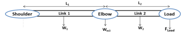
Figure 4: Free body diagram of the robotic arm in the fully stretched out configuration
