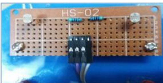
Fig 5: The photocell sensor board.
