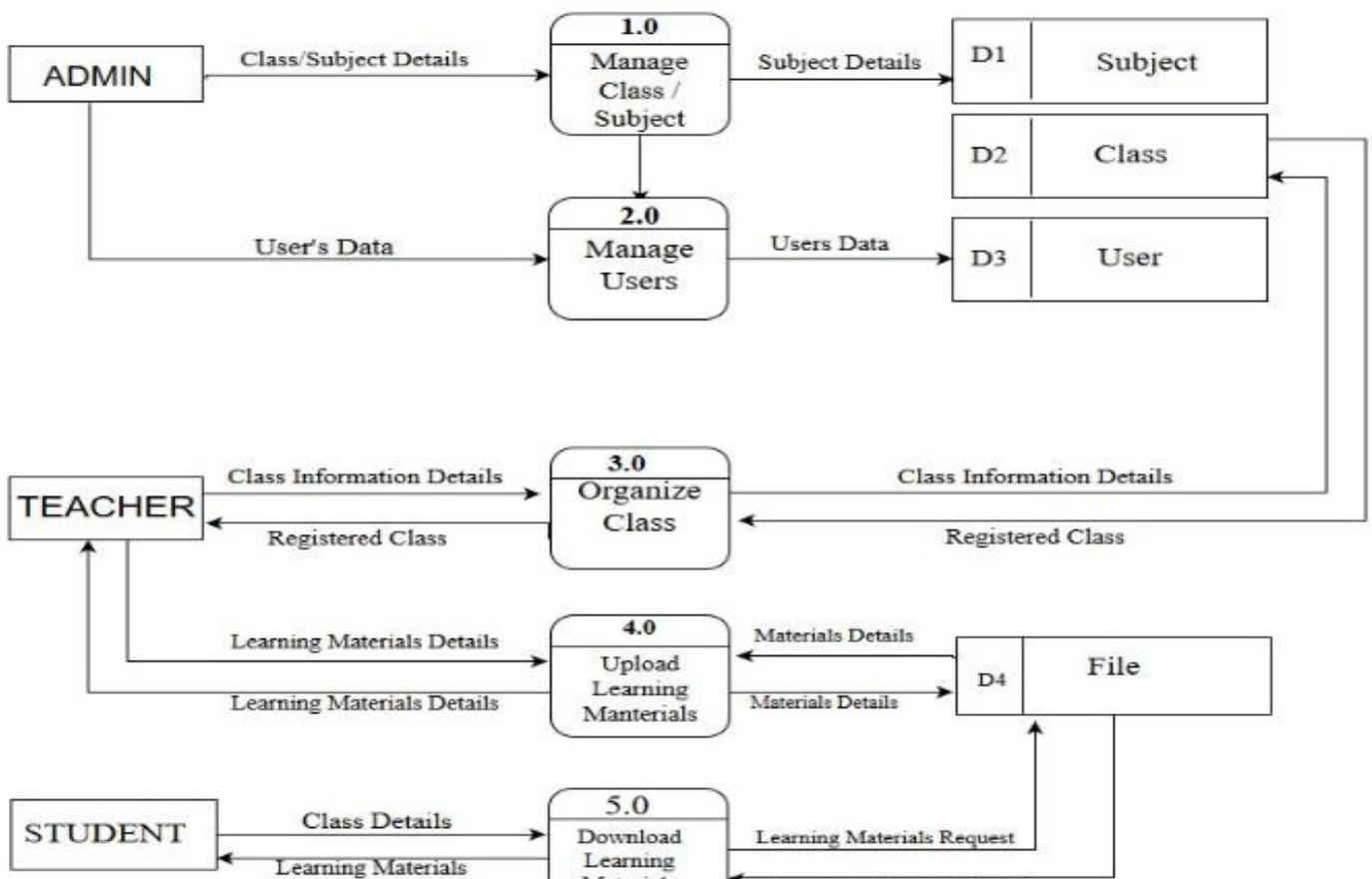
Fig 1: Showing LMS Dataflow Diagram
