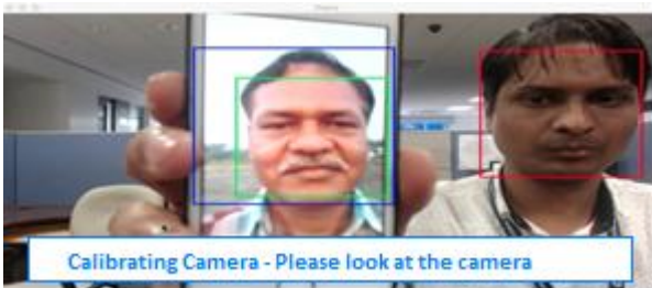
Fig 1: Application Screen with 2 faces, 1 st in and 2 nd out of the boundary
