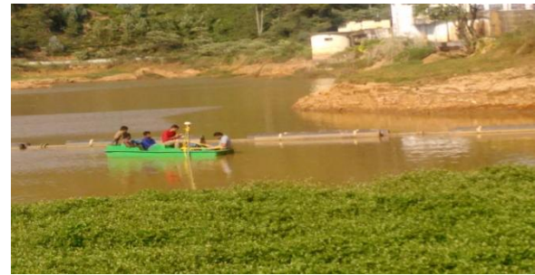
Figure 1: Boat with GPS Antenna & Echo-sounder (IBS Equipment)
