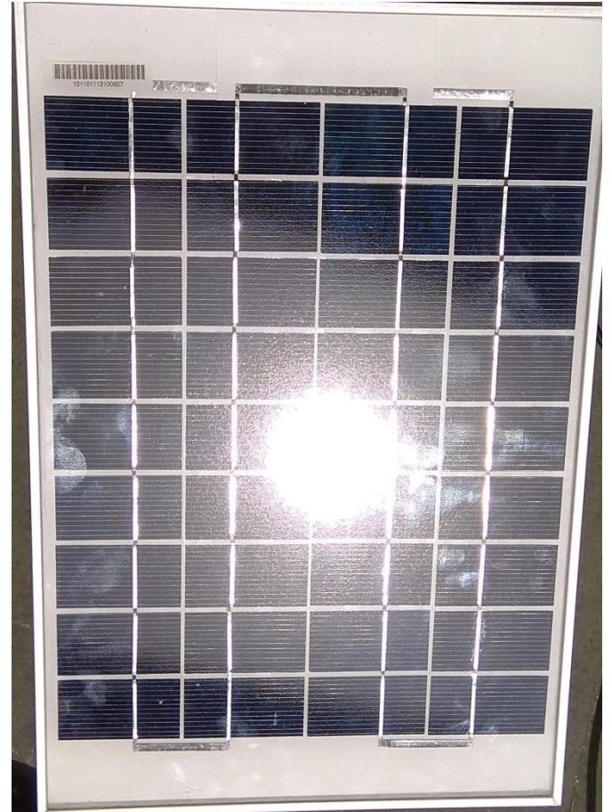
Fig 3: 11W 17V Solar Panel at 90° to sun
