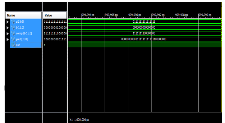
Fig. 2: Output stimulation of Radix-8 multiplier
