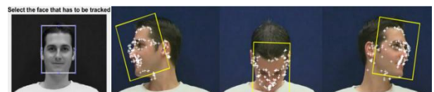
Fig 12: Outcome of the work in literature [27]; showing the result (face selection and tracking) of single face, 363 frames video sequence mcm0_head.mpg with frames #01, #38, #196 and #123 displayed.
