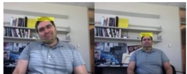
Fig 10: Outcome of the work in literature [25]; showing the tracking result of single face, 413 frames video sequence tilted_face.avi with frames #72 and #198 displayed.
