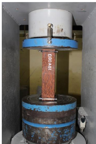
Fig.5 Compressive strength test of wood coconut sample
