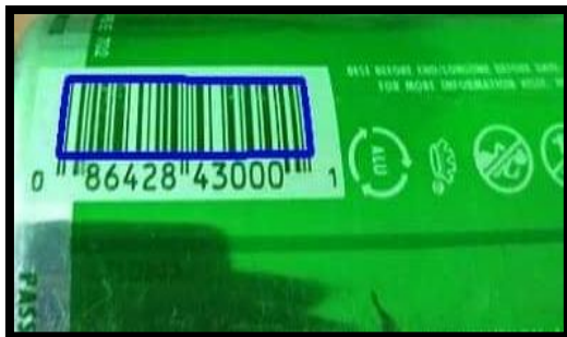
Fig.8: Angle invariant barcode detection
