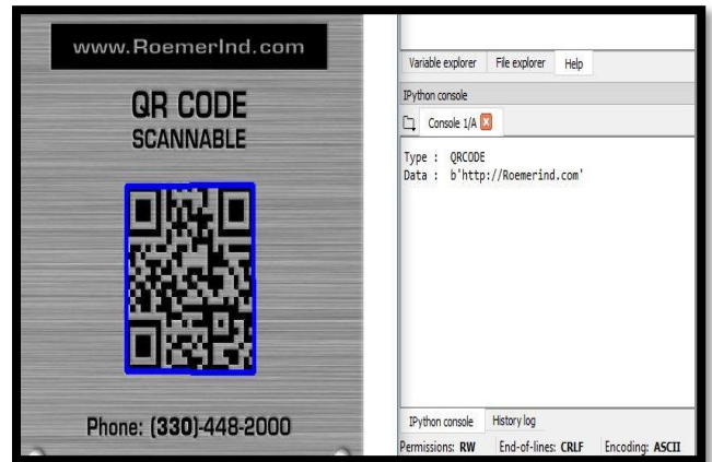
Fig.11: Detecting and decoding single 2D barcode from an image
