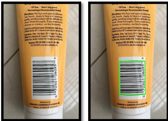
Fig.4: Single barcode detection from an image
