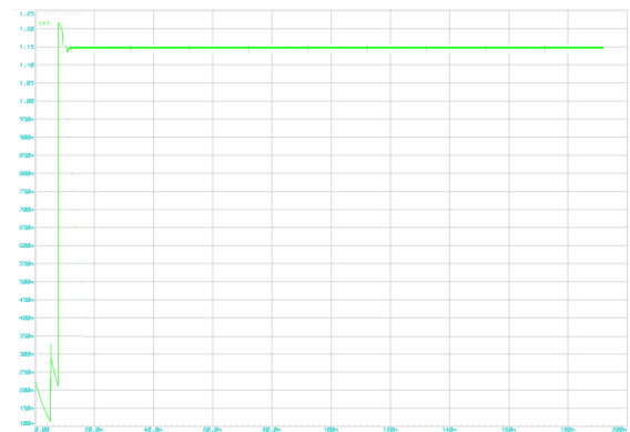
Fig.3 Battery charging current characteristics
