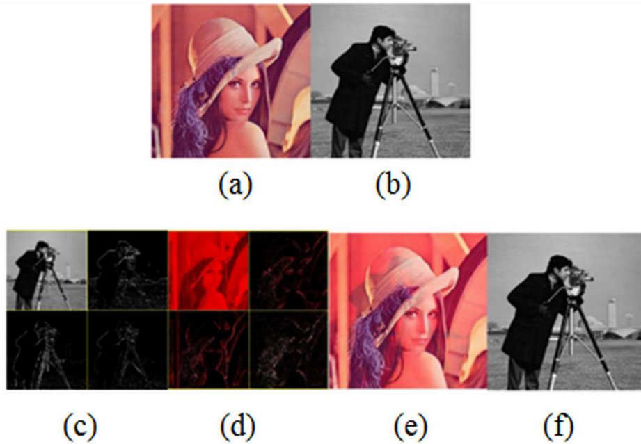
Fig 5: Results of IWT-DWT, (a) Cover Image, (b) Secret image, (c) IWT of Secret Image, (d) DWT of Cover Image, (e) Stego Image, (f) Extracted Image
