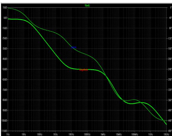
Fig 11: Frequency response of proposed buffer amplifier.
