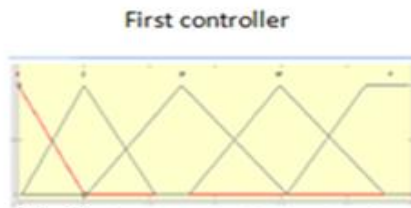
Fig.10 Input membership function for first controller voltage error
