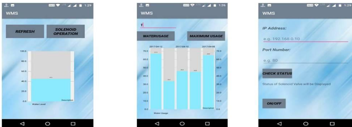
Fig. 3: Android application to view water level in the tank (left), to view water usage of a particular flat (middle), to control the solenoidal valve (right) [4]
