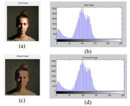
Fig. 4 (a) Original image (b) The histogram of the original image (c) Image obtain after AHE (d) The histogram after enhancement (AHE)
