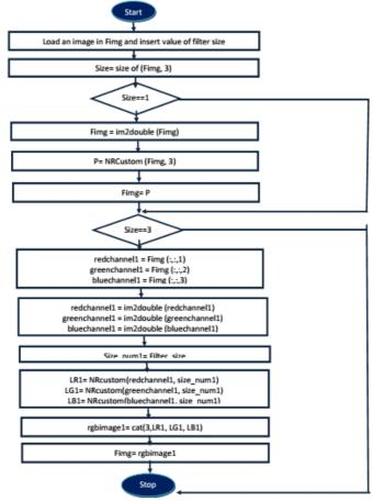
Fig. 6 Flow chart demonstrates the custom designed filter.
