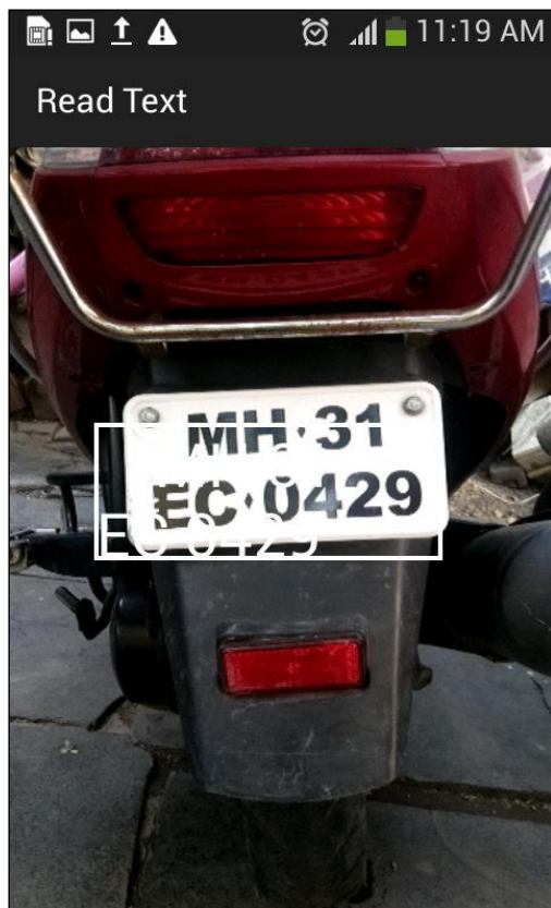
Fig 5: Vehicle Number Plate Detection
