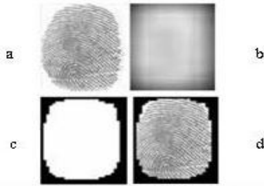
Figure 5: Different stages of Segmentation (a). Original image (b) Coherence image (c) Segmentation Mask (d) segmented image
