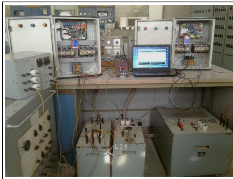
Fig 12: Experiment for the load balancing system with two control panels and one base station unit.
