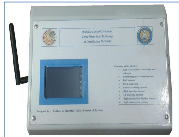
Fig 2: The smart energy meter
