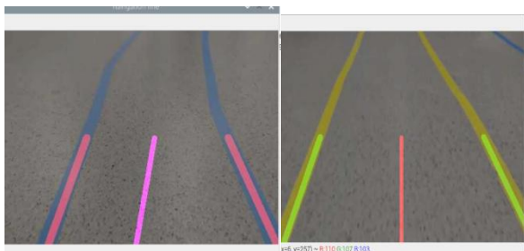
Figure 2: Detected Lane lines using conventional image processing algorithm.
