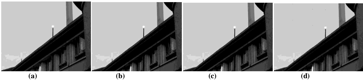
Figure 15: Application of the WF-LMS-MDBUTMF in de-noising salt and pepper noise from physics department (a) original image, (b) outcome of WF-MDBUTMF for 20% salt & pepper noise, (c) outcome of WF-MDBUTMF for 40% salt & pepper noise and (d) outcome of WF-MDBUTMF for 60% salt & pepper noise
