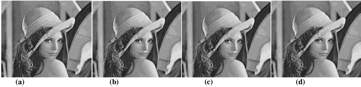
Figure 12: Application of WF-LMS-MDBUTMF in de-noising salt and pepper noise from Lena (a) original image, (b) outcome of WF-MDBUTMF for 20% salt & pepper noise, (c) outcome of WF-MDBUTMF for 40% salt & pepper noise (d) outcome of WF-MDBUTMF for 60% salt & pepper noise
