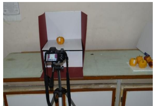
Figure 3: Imaging System for capturing Images of apple fruit
