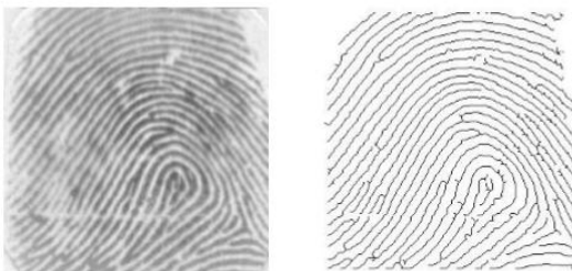
Fig 2: Original image (left) and the thinned image (right)
