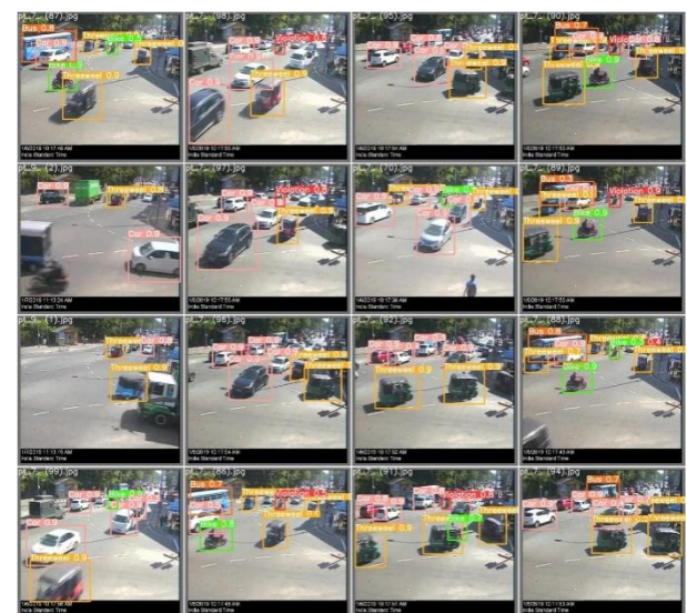
Fig 4: Object detection results for a white line violation
