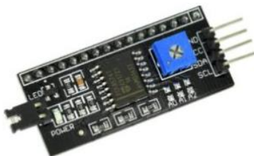
Figure 5. LCD I2C Module
