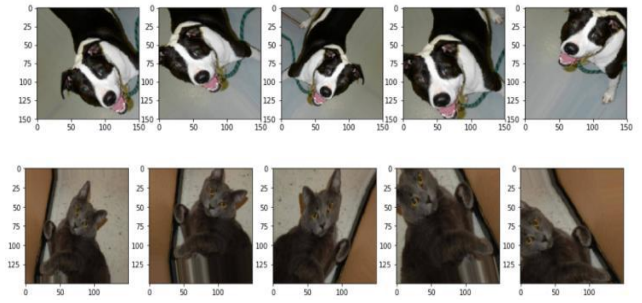
Figure 9: Examples of an Images are populated with zoom, rotation, height, width after applying ImageDataGenerator ().
