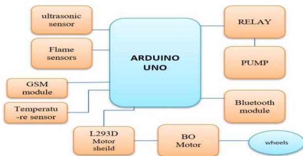
Figure 1: Block diagram of Fire Fighting Robot
