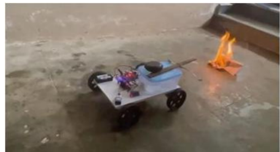
Figure 4: Extinguishing fire using fire fighting robot
