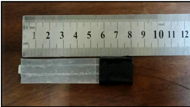
Figure 4: SMA Wire Embedded in Actuator
