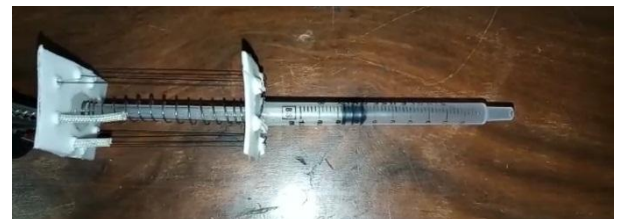
Fig 6: Single wire four loop configuration pump before actuation
