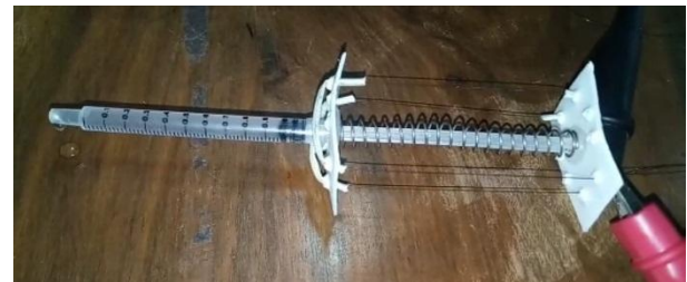
Fig 5: Two wire two loop configuration pump after actuation
