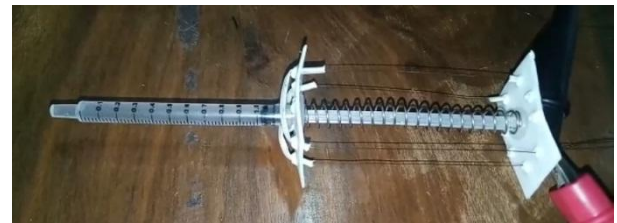
Fig 4: Two wire two loop configuration pump before actuation
