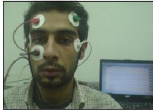
Fig 2: Installing electrodes for EOG signal acquisition
