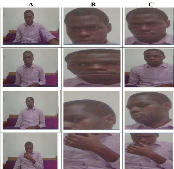
Fig. 4. Moving Object Detection and extraction, column A: input frame, column: B moving object extraction using ViBE, column C: moving object using EFF-ViBE
