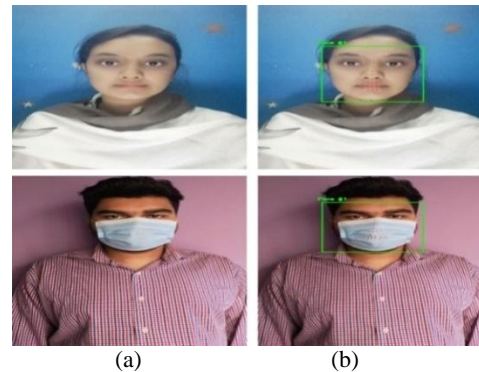
Fig. 3. Processing example of face detection for (non-mask and mask): a) input image, b) Face detection with landmark.
