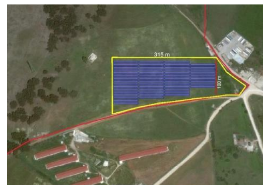
Fig 2: Solar panels installation design
