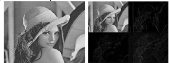
Fig 1.13: Example of 2-D Haar DWT.
