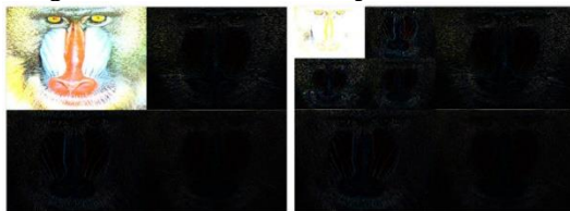
Fig 1.10: Example of 1 st and 2 nd level DWT decomposition.
