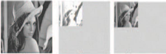
(a) Original image (b) 1 st level DWT (c) 2 nd level IWT Fig 1.15: Example of Integer Wavelet Transform in sub band LL.
