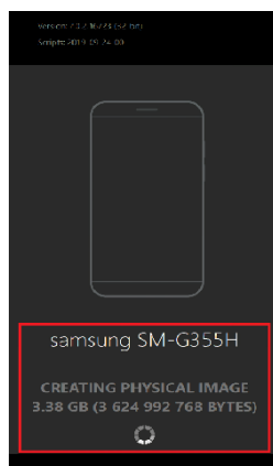
Figure 15. Process of Creating a Physical Image in MOBILedit Forensic
