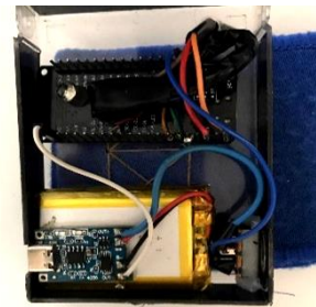
Figure 5: Connected microcontrollers to the wearable alert notification
