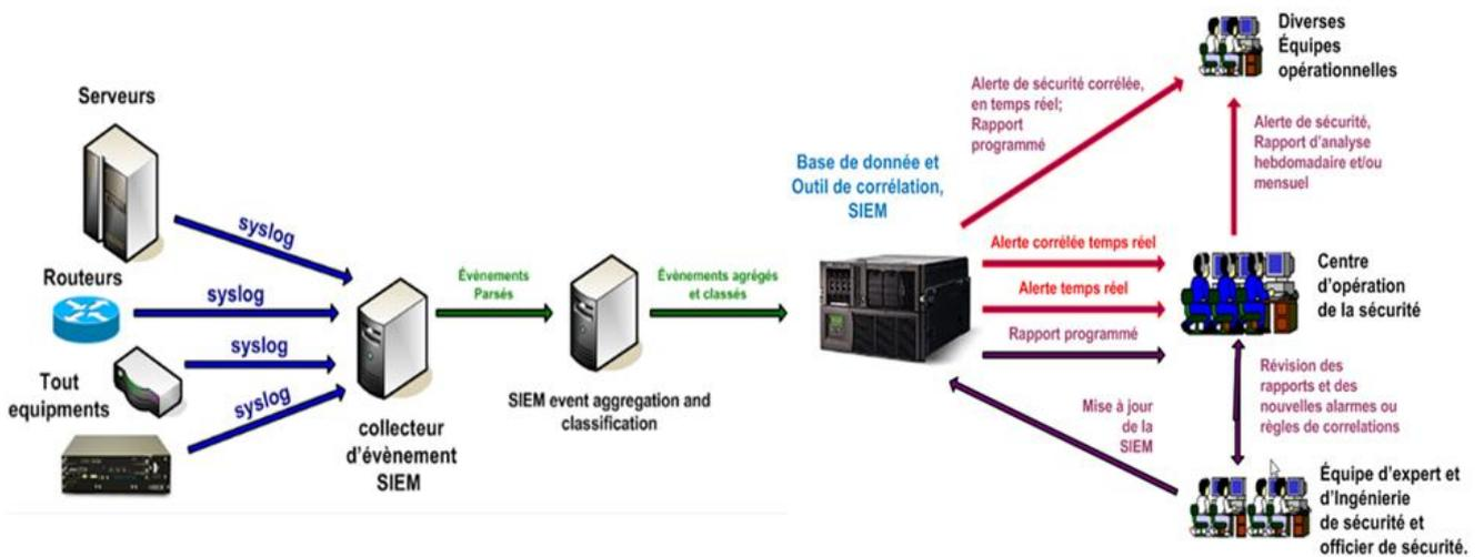
Figure 4: Principle of SEIM operation.
