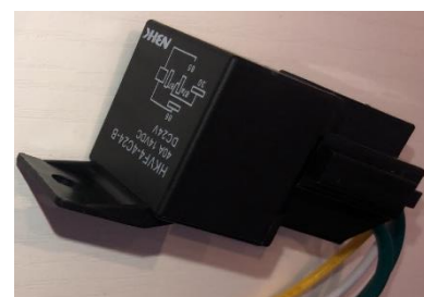
Figure 2 A 24 Volt Relay
