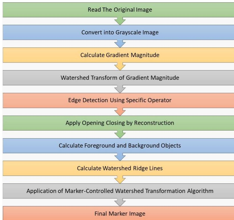
**Fig 2: Flowchart of the Marker-Controlled Watershed approach**
